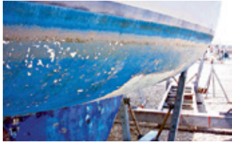
Paint blisters and lifts
